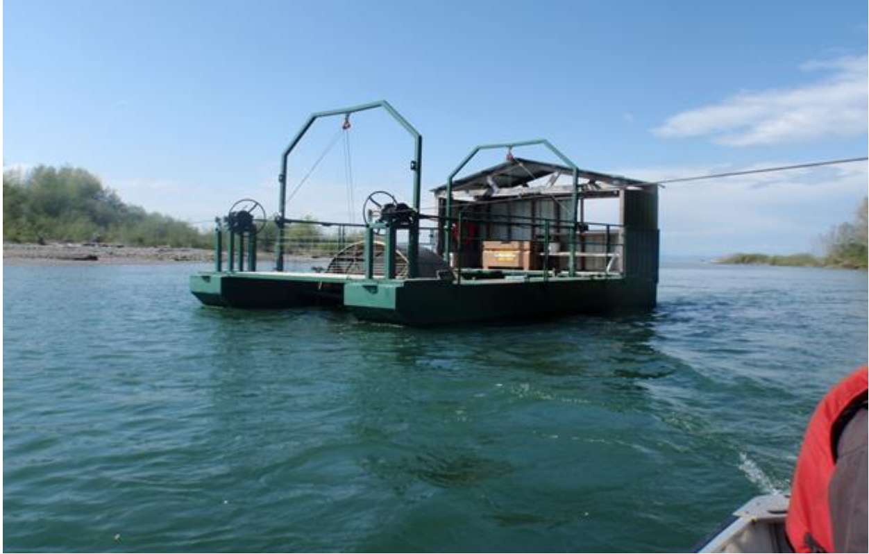
Figure 2. Elwha River 8' rotary screw trap fishing at Rkm 0.3 during the spring of 2010.
